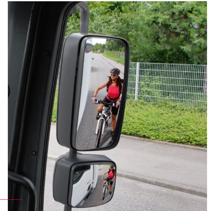
Mirror concept with large field of vision
