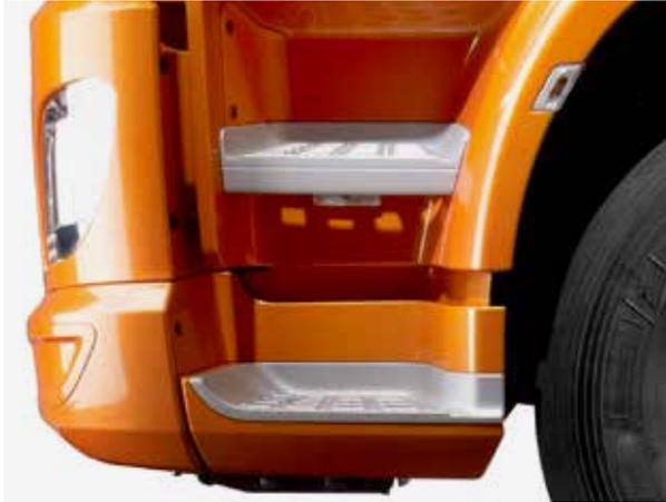
**ACCESSIBLE** Easy cab entry and exit is important for a truck in this class. The practical, low cab floor is only 1.18 m high on versions with the PACCAR MX 11 engine and 1.25 m high in the versions with PACCAR MX-13 engine. As a result, two or three steps are adequate. The aluminum steps are non-slip. That is safe, looks good and helps to prevent damage.
