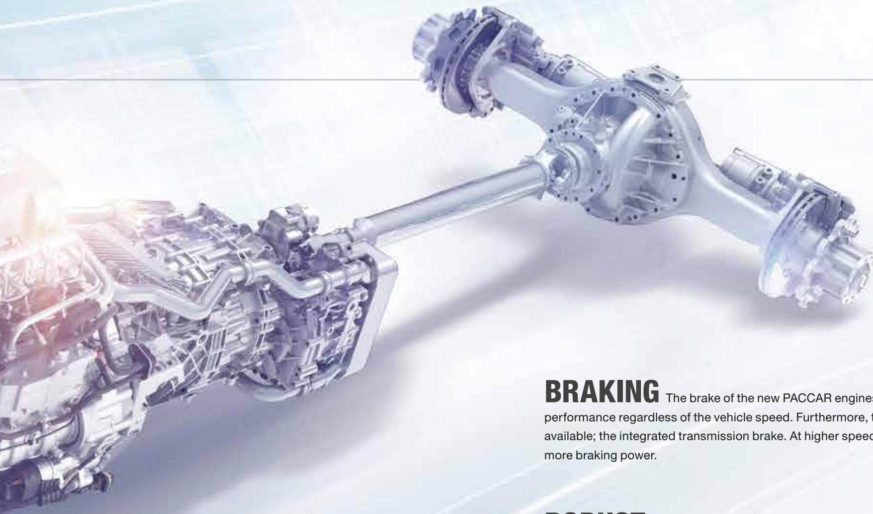
**BRAKING** The brake of the new PACCAR engines delivers impressive braking performance regardless of the vehicle speed. Furthermore, the new Intarder 3 is available; the integrated transmission brake. At higher speeds, it offers the driver even more braking power.
