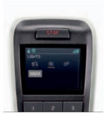
Turn the lights on. Do you have work lights, beacons or specific lights from the bodybuilder? Use the Work Remote to switch them on or off.
