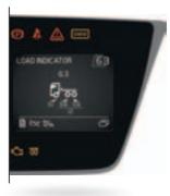
**LOAD INDICATOR** The enhanced load indicator allows you to precisely monitor axle load.
