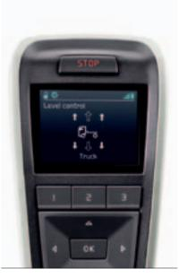
Balance it all with your fingertips. Cut the wire. With the Work Remote in your hand, you can control the air suspension manually while walking around freely.
